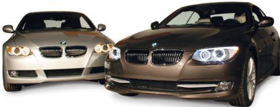
E92/E93 comparison: Predecessor at left, SA 5AK LED light elements at right and top
